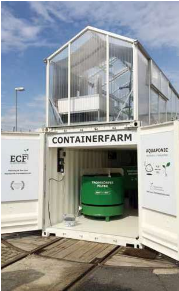
Prototype of container farm tested by Efficient City Farming (ECF) with aquaculture in container and hydroponics in greenhouse.
