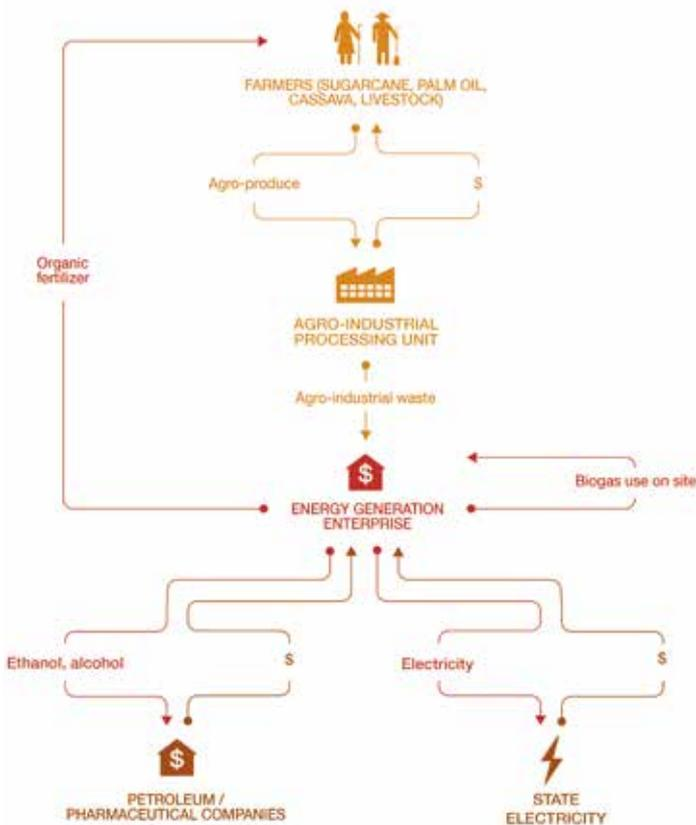
Figure 2. Process flow for on-site energy generation by agro-industries (Otto and Drechsel, 2017)
