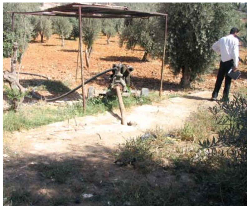
The water is pumped out of the ditches on the fields Photo: Sahar Dalahmeh
