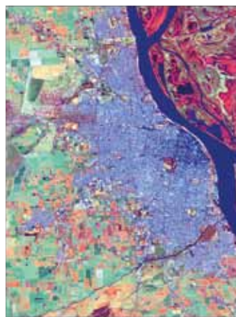
Landsat 8/NASA Multispectral Image. The blue band is the Paraná river and the pink/ reddish colours correspond to the islands of the Paraná delta. The periurban zone corresponds to the areas with green color (cultivated area) and brown color (non-cultivated areas).
