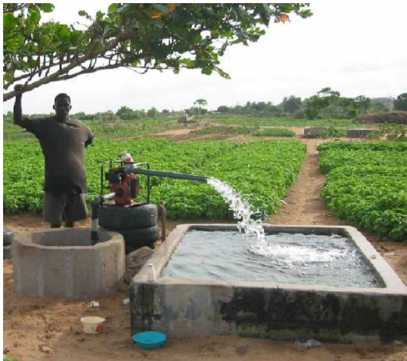
Figure 8.3: Watering can irrigation with well and storage reservoirs in Togo. Further reservoirs are visible in the background.
